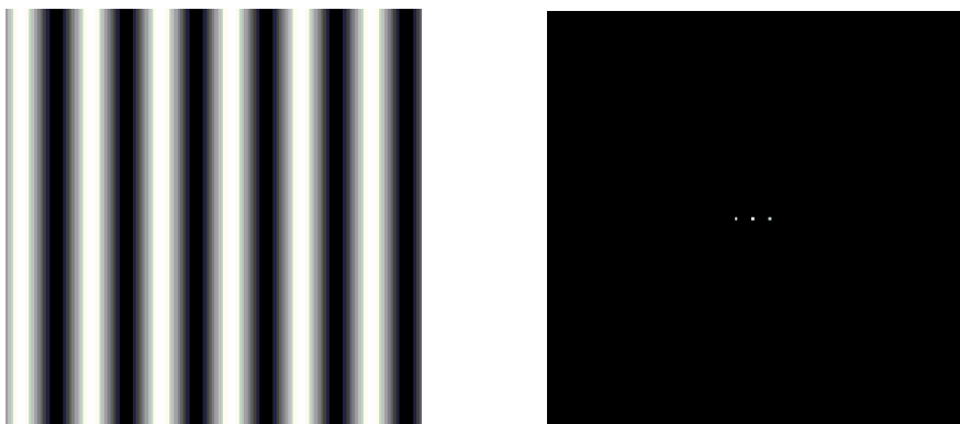
Figure 9: Image of f(x, y) = \text{sen}\left(\frac{2\pi x}{T}\right) with T = 100 and x = 1, 2, \dots, 600 , and its Fourier spectrum.
