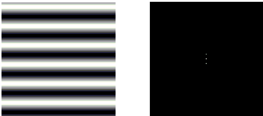
Figure 8: Image of f(x, y) = \text{sen}\left(\frac{2\pi y}{T}\right) with T = 100 and y = 1, 2, \dots, 600 , and its Fourier spectrum.
